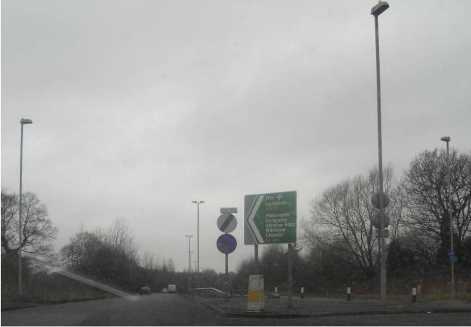
The Styal Road Junction uses Iridium lanterns manufactured by Philips Lighting (see photo below). These are mounted at 10m, with a 0.5m outreach bracket and utilise high pressure sodium lamps which are likely to be either 150watt or 250watt High Pressure Sodium (SONT-P Plus Pia) lamps.
